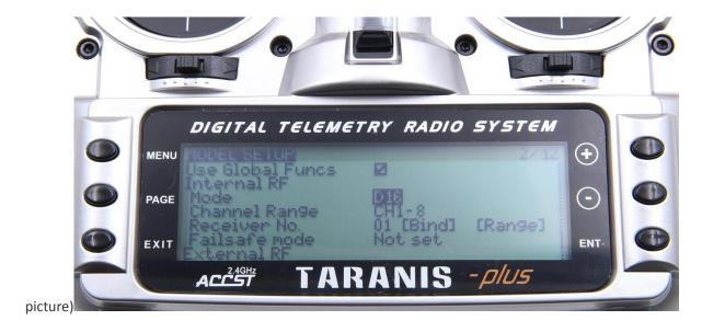
lacktriangle 2: Move the cursor to the "Mode" option , "Mode" option t he working mode of XJT can be switched. There are three types of D16, D8, and LR12 respectively. Please select according to your receiver:
